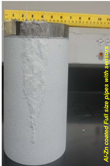
Wear Test on Corroded samples
